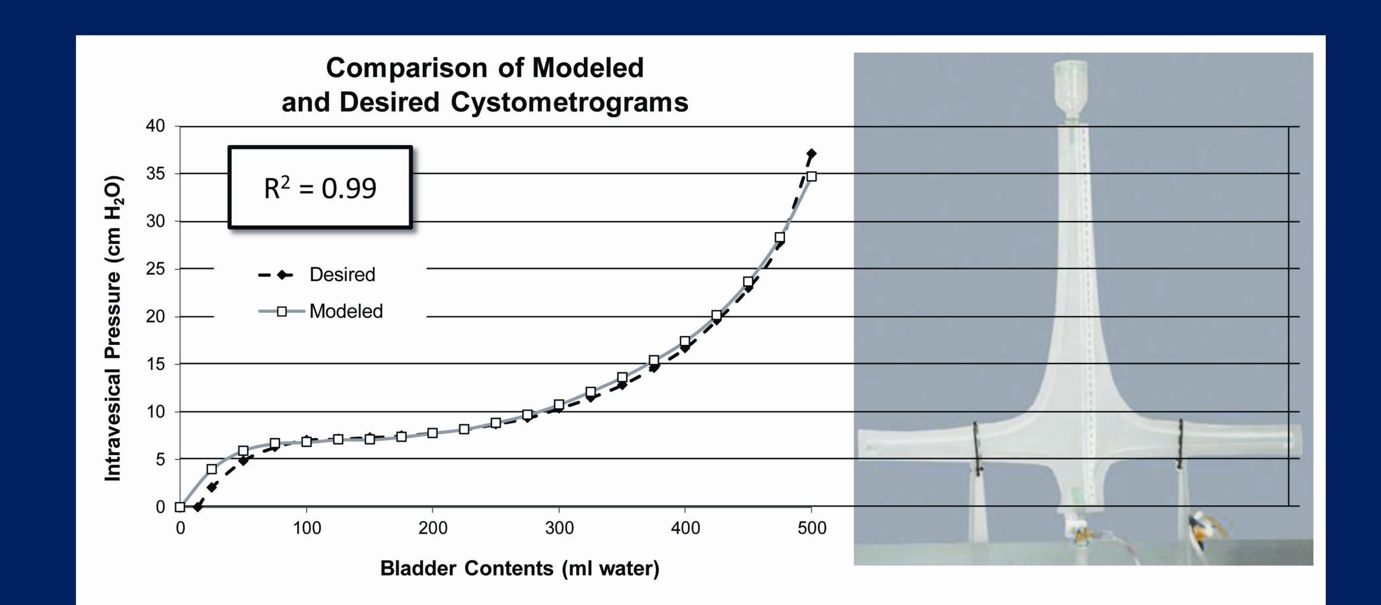
The constructed bladder model has a pressure volume curve very similar (R<sup>2</sup> 0.99) to the desired values, between 25 and 500 ml.
