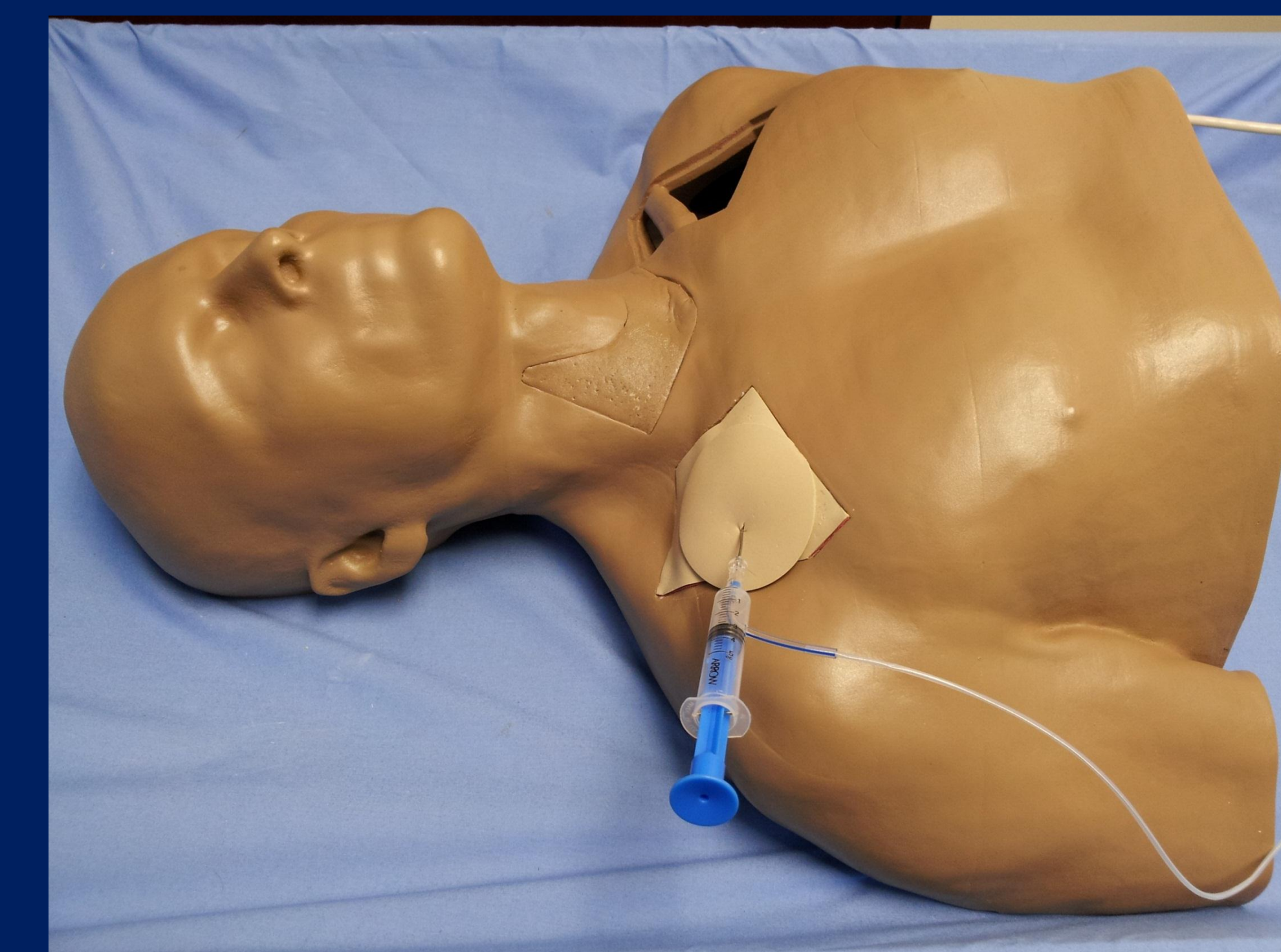
Figure 1. The mixed reality central venous access simulator; a needle (tracked in 3D space) is inserted via the skin patch to access the subclavian vein
