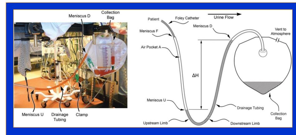
**Figure 2:** A photograph and schematic depiction of a urinary catheter drainage system which demonstrates how a dependent loop in the drainage tubing will result in a trapped air volume on the patient side of the loop. The meniscus height differential will act as a U-tube manometer in this scenario and provide an accurate measure of pressure in the trapped air space and thus back pressure into the patient's bladder.
