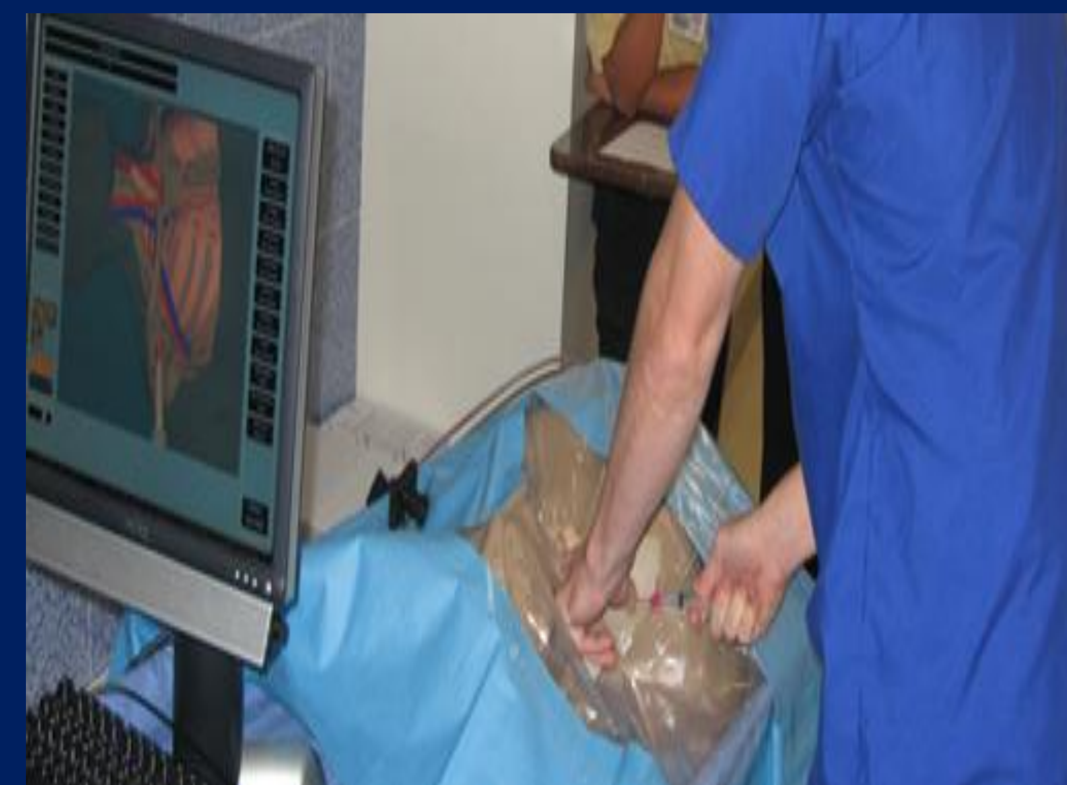
Figure 1: The subclavian central venous access mixed reality simulator records and analyzes the placement of the needle
