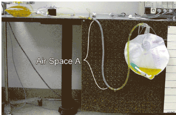
Figure 1: In vitro model of urinary system, Foley catheter, drainage tube and collection bag
